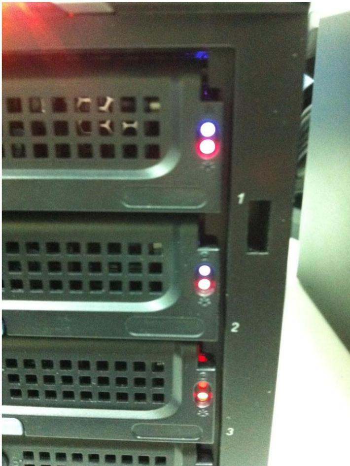
And after several seconds, we can observe that the system is rebuilding bootos and RAID from Intel® Rapid Storage Tool. It may take 24 hours to rebuild the RAID. At first, we can see the Storage shows red in VMS panel.
